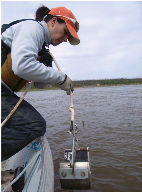
Using a Petite Ponar, a type of grab sampler, to collect mud with benthos in offshore areas
