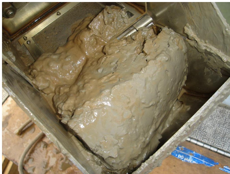
Photo 2-4. Example of a clay substrate Ponar grab sample on Assean Lake.
