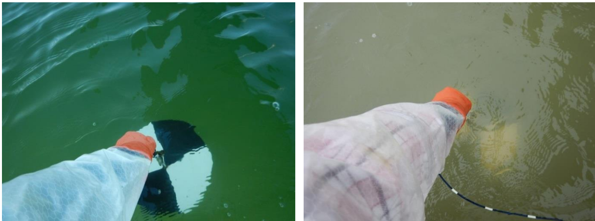
Measuring Secchi disk depth in Cormorant Lake (left) and Stephens Lake (right).
