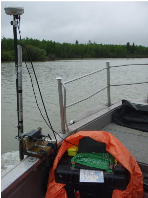
Hydroacoustic sampling on Cross Lake.
