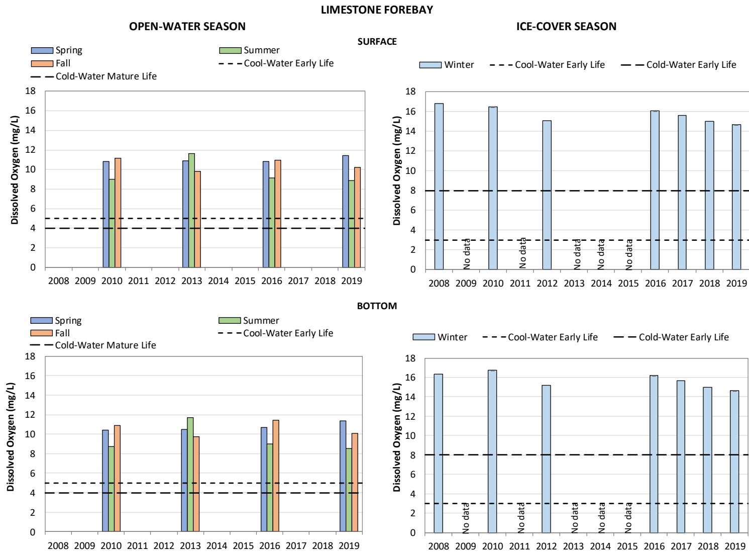
Figure 3.2-14. 2008-2019 Limestone Forebay surface and bottom dissolved oxygen concentrations with comparison to instantaneous minimum objectives for the protection of aquatic life.
