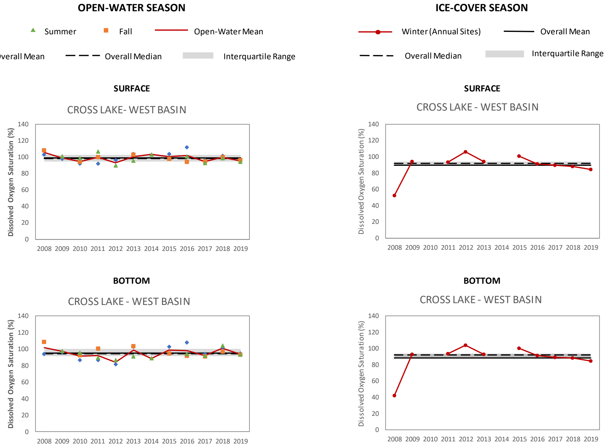
Figure 3.2-14. 2008-2019 Cross Lake open-water season and ice-cover season surface and bottom dissolved oxygen saturation.
