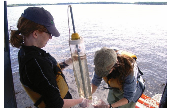
Water quality sampling using a Kemmerer sampler
